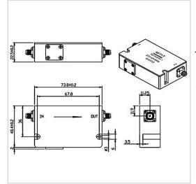
RF Solution offer a wide selection of Dual Junction Isolator for global customers. TG7448HS is a Dual Junction Isolator in Frequency Range of 700~4200 MHz. It is made of high quality materials under a high standard, the Bandwidth Max of this product is 5~20%, Insertion Loss Max is 0.40~1.40 dB and Isolation Min is 34.0~46.0 dB. The component has a good working performance and stability, it is ideal for handling a Forward Power of 100/200/300 W.
