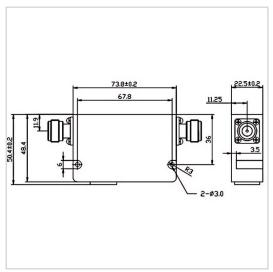
RF Solution offer a wide selection of Dual Junction Isolator for global customers. TG7448HN is a Dual Junction Isolator in Frequency Range of  $700\sim4200$  MHz. It is made of high quality materials under a high standard, the Bandwidth Max of this product is  $5\sim20\%$ , Insertion Loss Max is  $0.40\sim1.20$  dB and Isolation Min is  $36.0\sim50.0$  dB. The component has a good working performance and stability, it is ideal for handling a Forward Power of 300 W.
