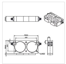
RF Solution offer a wide selection of Dual Junction Isolator for global customers. TG7038XS is a Dual Junction Isolator in Frequency Range of  $300\sim1850$  MHz. It is made of high quality materials under a high standard, the Bandwidth Max of this product is  $5\sim20\%$ , Insertion Loss Max is  $0.40\sim1.60$  dB and Isolation Min is  $32.0\sim50.0$  dB. The component has a good working performance and stability, it is ideal for handling a Forward Power of 100~W.
