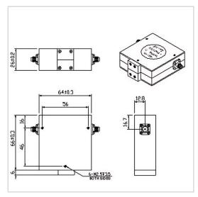
RF Solution offer a wide selection of Coaxial Isolator for global customers. TG6466KS is a Coaxial Isolator in Frequency Range of  $0.95\sim2.0$  GHz. It is made of high quality materials under a high standard, the Bandwidth Max of this product is 100%, Insertion Loss Max is  $0.70\sim0.80$  dB and Isolation Min is  $16.0\sim17.0$  dB. The component has a good working performance and stability, it is ideal for handling a Forward Power of 100 W.
