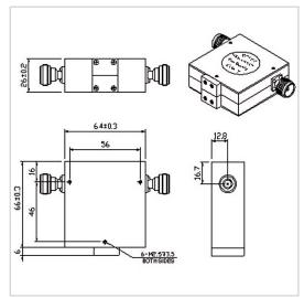
RF Solution offer a wide selection of Coaxial Isolator for global customers. TG6466KN is a Coaxial Isolator in Frequency Range of  $0.95\sim2.0$  GHz. It is made of high quality materials under a high standard, the Bandwidth Max of this product is 100%, Insertion Loss Max is  $0.70\sim0.80$  dB and Isolation Min is  $16.0\sim17.0$  dB. The component has a good working performance and stability, it is ideal for handling a Forward Power of 150 W.
