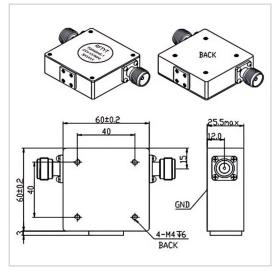
RF Solution offer a wide selection of Coaxial Isolator for global customers. TG6466HN is a Coaxial Isolator in Frequency Range of 30~40 MHz. It is made of high quality materials under a high standard, the Bandwidth Max of this product is 5%, Insertion Loss Max is 1.50~2.00 dB and Isolation Min is 18.0~20.0 dB. The component has a good working performance and stability, it is ideal for handling a Forward Power of 50 W.
