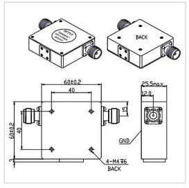
RF Solution offer a wide selection of Coaxial Isolator for global customers. TG6466ES is a Coaxial Isolator in Frequency Range of 100~200 MHz. It is made of high quality materials under a high standard, the Bandwidth Max of this product is 20%, Insertion Loss Max is 0.45~0.80 dB and Isolation Min is 18.0~23.0 dB. The component has a good working performance and stability, it is ideal for handling a Forward Power of 100 W.
