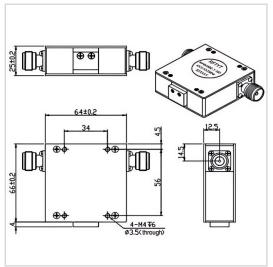
RF Solution offer a wide selection of Coaxial Isolator for global customers. TG6466EN is a Coaxial Isolator in Frequency Range of 100~200 MHz. It is made of high quality materials under a high standard, the Bandwidth Max of this product is 5%, Insertion Loss Max is  $0.45\sim0.70$  dB and Isolation Min is  $18.0\sim23.0$ dB. The component has a good working performance and stability, it is ideal for handling a Forward Power of 300 W.
