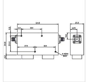
RF Solution offer a wide selection of Dual Junction Isolator for global customers. TG6434AS is a Dual Junction Isolator in Frequency Range of 2.0~4.0 GHz. It is made of high quality materials under a high standard, the Bandwidth Max of this product is 100%, Insertion Loss Max is 0.80~1.00 dB and Isolation Min is 36.0~40.0 dB. The component has a good working performance and stability, it is ideal for handling a Forward Power of 100 W.
