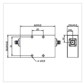
RF Solution offer a wide selection of Coaxial Isolator for global customers. TG6237AS is a Coaxial Isolator in Frequency Range of 2.0~8.0 GHz. It is made of high quality materials under a high standard, the Bandwidth Max of this product is 100%, Insertion Loss Max is 1.20~1.70 dB and Isolation Min is 13.0~15.0 dB. The component has a good working performance and stability, it is ideal for handling a Forward Power of 20 W.
