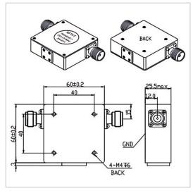
RF Solution offer a wide selection of Coaxial Isolator for global customers. TG6060EN is a Coaxial Isolator in Frequency Range of 40~400 MHz. It is made of high quality materials under a high standard, the Bandwidth Max of this product is 50%, Insertion Loss Max is  $0.40 \sim 1.80$  dB and Isolation Min is  $18.0 \sim 23.0$ dB. The component has a good working performance and stability, it is ideal for handling a Forward Power of 50/100 W.
