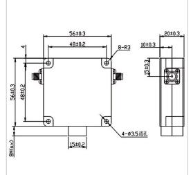
RF Solution offer a wide selection of Broadband Isolator for global customers. TG5656AS is a Broadband Isolator in Frequency Range of 0.8~2.0 GHz. It is made of high quality materials under a high standard, the Bandwidth Max of this product is 100%, Insertion Loss Max is 1.2 dB and Isolation Min is 13.0 dB. The component has a good working performance and stability, it is ideal for handling a Forward Power of 50 W.
