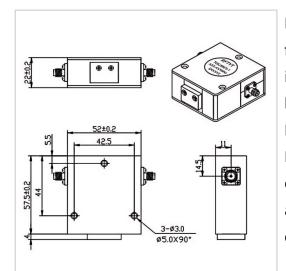
RF Solution offer a wide selection of Coaxial Isolator for global customers. TG5258ES is a Coaxial Isolator in Frequency Range of 150~330 MHz. It is made of high quality materials under a high standard, the Bandwidth Max of this product is 20%, Insertion Loss Max is 0.30~0.90 dB and Isolation Min is 18.0~23.0 dB. The component has a good working performance and stability, it is ideal for handling a Forward Power of 100 W.
