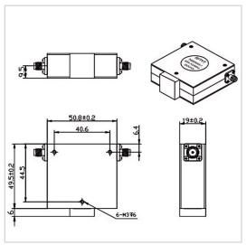
RF Solution offer a wide selection of Coaxial Isolator for global customers. TG5050AS is a Coaxial Isolator in Frequency Range of  $1.25\sim3.0$  GHz. It is made of high quality materials under a high standard, the Bandwidth Max of this product is 100%, Insertion Loss Max is  $0.50\sim0.80$  dB and Isolation Min is  $16.0\sim18.0$  dB. The component has a good working performance and stability, it is ideal for handling a Forward Power of  $100\ W$ .
