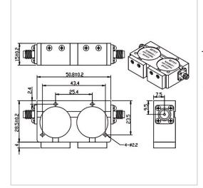
RF Solution offer a wide selection of Dual Junction Isolator for global customers. TG5028XS is a Dual Junction Isolator in Frequency Range of 700~4200 MHz. It is made of high quality materials under a high standard, the Bandwidth Max of this product is 5~20%, Insertion Loss Max is 0.60~1.20 dB and Isolation Min is 34.0~100.0 dB. The component has a good working performance and stability, it is ideal for handling a Forward Power of 100 W.
