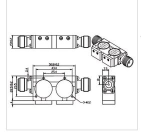
RF Solution offer a wide selection of Dual Junction Isolator for global customers. TG5028XN is a Dual Junction Isolator in Frequency Range of 700~4200 MHz. It is made of high quality materials under a high standard, the Bandwidth Max of this product is 5~20%, Insertion Loss Max is 0.60~1.20 dB and Isolation Min is 34.0~100.0 dB. The component has a good working performance and stability, it is ideal for handling a Forward Power of 100 W.
