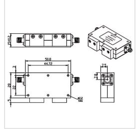
RF Solution offer a wide selection of Dual Junction Isolator for global customers. TG5028CS is a Dual Junction Isolator in Frequency Range of 3.0~6.0 GHz. It is made of high quality materials under a high standard, the Bandwidth Max of this product is 100%, Insertion Loss Max is 0.60~1.00 dB and Isolation Min is 36.0~40.0 dB. The component has a good working performance and stability, it is ideal for handling a Forward Power of 100 W.
