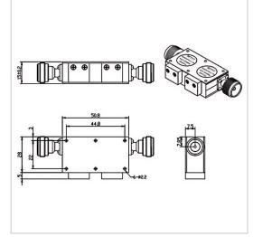
RF Solution offer a wide selection of Dual Junction Isolator for global customers. TG5028CN is a Dual Junction Isolator in Frequency Range of 3.0~6.0 GHz. It is made of high quality materials under a high standard, the Bandwidth Max of this product is 100%, Insertion Loss Max is 0.60~1.00 dB and Isolation Min is 36.0~40.0 dB. The component has a good working performance and stability, it is ideal for handling a Forward Power of 100 W.
