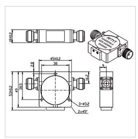
RF Solution offer a wide selection of Coaxial Isolator for global customers. TG4550XN is a Coaxial Isolator in Frequency Range of 250~1400 MHz. It is made of high quality materials under a high standard, the Bandwidth Max of this product is 40%, Insertion Loss Max is 0.25~0.90 dB and Isolation Min is 15.0~23.0 dB. The component has a good working performance and stability, it is ideal for handling a Forward Power of 100 W.
