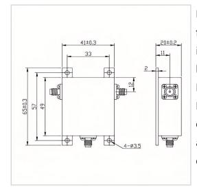
RF Solution offer a wide selection of Coaxial Isolator for global customers. TG4149AS is a Coaxial Isolator in Frequency Range of 300~1000 MHz. It is made of high quality materials under a high standard, the Bandwidth Max of this product is 50%, Insertion Loss Max is 0.80~1.20 dB and Isolation Min is 14.0~20.0 dB. The component has a good working performance and stability, it is ideal for handling a Forward Power of 30 W.
