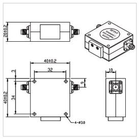
RF Solution offer a wide selection of Coaxial Isolator for global customers. TG4040AS is a Coaxial Isolator in Frequency Range of 1.50~3.0 GHz. It is made of high quality materials under a high standard, the Bandwidth Max of this product is 100%, Insertion Loss Max is 0.50~0.60 dB and Isolation Min is 17.0~18.0 dB. The component has a good working performance and stability, it is ideal for handling a Forward Power of 100 W.
