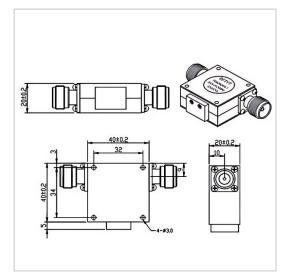
RF Solution offer a wide selection of Coaxial Isolator for global customers. TG4040AN is a Coaxial Isolator in Frequency Range of 1.5~3.0 GHz. It is made of high quality materials under a high standard, the Bandwidth Max of this product is 100%, Insertion Loss Max is 0.50~0.60 dB and Isolation Min is 17.0~18.0 dB. The component has a good working performance and stability, it is ideal for handling a Forward Power of 100 W.
