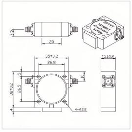
RF Solution offer a wide selection of Coaxial Isolator for global customers. TG3538XS is a Coaxial Isolator in Frequency Range of 300~1800 MHz. It is made of high quality materials under a high standard, the Bandwidth Max of this product is 30%, Insertion Loss Max is 0.20~0.80 dB and Isolation Min is 16.0~25.0 dB. The component has a good working performance and stability, it is ideal for handling a Forward Power of 150 W.
