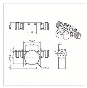
RF Solution offer a wide selection of Coaxial Isolator for global customers. TG3538XN is a Coaxial Isolator in Frequency Range of 300~1800 MHz. It is made of high quality materials under a high standard, the Bandwidth Max of this product is 30%, Insertion Loss Max is 0.20~0.70 dB and Isolation Min is 17.0~25.0 dB. The component has a good working performance and stability, it is ideal for handling a Forward Power of 100 W.
