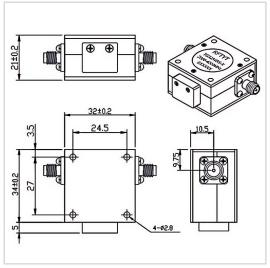
RF Solution offer a wide selection of Coaxial Isolator for global customers. TG3234BS is a Coaxial Isolator in Frequency Range of  $2.0{\sim}4.0$  GHz. It is made of high quality materials under a high standard, the Bandwidth Max of this product is 100%, Insertion Loss Max is  $0.40{\sim}0.50$  dB and Isolation Min is  $18.0{\sim}20.0$  dB. The component has a good working performance and stability, it is ideal for handling a Forward Power of 100 W.
