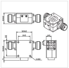
RF Solution offer a wide selection of Coaxial Isolator for global customers. TG3234BN is a Coaxial Isolator in Frequency Range of 2.0~4.0 GHz. It is made of high quality materials under a high standard, the Bandwidth Max of this product is 100%, Insertion Loss Max is 0.50~0.60 dB and Isolation Min is 18.0~19.0 dB. The component has a good working performance and stability, it is ideal for handling a Forward Power of 150 W.
