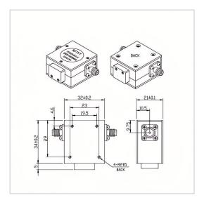
RF Solution offer a wide selection of Coaxial Isolator for global customers. TG3234AS is a Coaxial Isolator in Frequency Range of  $2.0{\sim}4.0$  GHz. It is made of high quality materials under a high standard, the Bandwidth Max of this product is 100%, Insertion Loss Max is  $0.40{\sim}0.50$  dB and Isolation Min is  $18.0{\sim}20.0$  dB. The component has a good working performance and stability, it is ideal for handling a Forward Power of 150 W.
