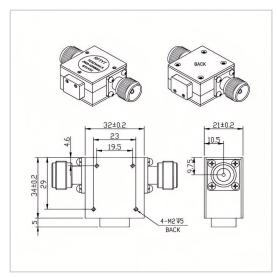
RF Solution offer a wide selection of Coaxial Isolator for global customers. TG3234AN is a Coaxial Isolator in Frequency Range of  $2.0{\sim}4.0$  GHz. It is made of high quality materials under a high standard, the Bandwidth Max of this product is 100%, Insertion Loss Max is  $0.40{\sim}0.50$  dB and Isolation Min is  $18.0{\sim}20.0$  dB. The component has a good working performance and stability, it is ideal for handling a Forward Power of 150 W.
