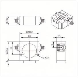
RF Solution offer a wide selection of Coaxial Isolator for global customers. TG3232XS is a Coaxial Isolator in Frequency Range of 700~3000 MHz. It is made of high quality materials under a high standard, the Bandwidth Max of this product is 25%, Insertion Loss Max is 0.30~0.60 dB and Isolation Min is 18.0~25.0 dB. The component has a good working performance and stability, it is ideal for handling a Forward Power of 150 W.
