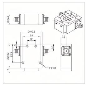
RF Solution offer a wide selection of Coaxial Isolator for global customers. TG3033XS is a Coaxial Isolator in Frequency Range of  $700\sim3000$  MHz. It is made of high quality materials under a high standard, the Bandwidth Max of this product is 25%, Insertion Loss Max is  $0.30\sim0.60$  dB and Isolation Min is  $16.0\sim23.0$  dB. The component has a good working performance and stability, it is ideal for handling a Forward Power of 150 W.
