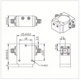
RF Solution offer a wide selection of Coaxial Isolator for global customers. TG2528XS is a Coaxial Isolator in Frequency Range of 700~5000 MHz. It is made of high quality materials under a high standard, the Bandwidth Max of this product is 25%, Insertion Loss Max is 0.30~0.60 dB and Isolation Min is 17.0~23.0 dB. The component has a good working performance and stability, it is ideal for handling a Forward Power of 150 W.
