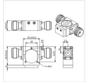
RF Solution offer a wide selection of Coaxial Isolator for global customers. TG2528XN is a Coaxial Isolator in Frequency Range of 700~5000 MHz. It is made of high quality materials under a high standard, the Bandwidth Max of this product is 25%, Insertion Loss Max is 0.30~0.60 dB and Isolation Min is 17.0~23.0 dB. The component has a good working performance and stability, it is ideal for handling a Forward Power of 150 W.
