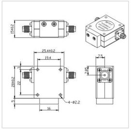
RF Solution offer a wide selection of Coaxial Isolator for global customers. TG2528CS is a Coaxial Isolator in Frequency Range of 3.0~6.0 GHz. It is made of high quality materials under a high standard, the Bandwidth Max of this product is 100%, Insertion Loss Max is 0.40~0.50 dB and Isolation Min is 18.0~20.0 dB. The component has a good working performance and stability, it is ideal for handling a Forward Power of 100 W.
