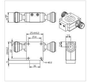
RF Solution offer a wide selection of Coaxial Isolator for global customers. TG2528CN is a Coaxial Isolator in Frequency Range of 3.0~6.0 GHz. It is made of high quality materials under a high standard, the Bandwidth Max of this product is 100%, Insertion Loss Max is 0.40~0.50 dB and Isolation Min is 18.0~20.0 dB. The component has a good working performance and stability, it is ideal for handling a Forward Power of 150 W.
