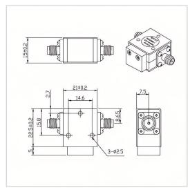
RF Solution offer a wide selection of Coaxial Isolator for global customers. TG2123BS is a Coaxial Isolator in Frequency Range of  $4.0 \sim 8.0$  GHz. It is made of high quality materials under a high standard, the Bandwidth Max of this product is 100%, Insertion Loss Max is  $0.40 \sim 0.60$  dB and Isolation Min is  $18.0 \sim 20.0$  dB. The component has a good working performance and stability, it is ideal for handling a Forward Power of 50 W.
