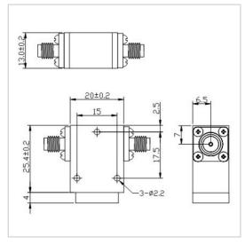
RF Solution offer a wide selection of Coaxial Isolator for global customers. TG2025XS is a Coaxial Isolator in Frequency Range of 900~5000 MHz. It is made of high quality materials under a high standard, the Bandwidth Max of this product is 20%, Insertion Loss Max is 0.25~0.50 dB and Isolation Min is 18.0~23.0 dB. The component has a good working performance and stability, it is ideal for handling a Forward Power of 100 W.
