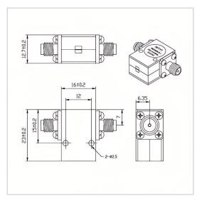
RF Solution offer a wide selection of Coaxial Isolator for global customers. TG1623CS is a Coaxial Isolator in Frequency Range of  $5.0\sim7.4$  GHz. It is made of high quality materials under a high standard, the Bandwidth Max of this product is 20%, Insertion Loss Max is  $0.40\sim0.50$  dB and Isolation Min is  $18.0\sim20.0$  dB. The component has a good working performance and stability, it is ideal for handling a Forward Power of 100 W.
