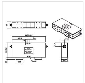
RF Solution offer a wide selection of Dual Junction Isolator for global customers. TG14566KS is a Dual Junction Isolator in Frequency Range of 1.0~2.0 GHz. It is made of high quality materials under a high standard, the Bandwidth Max of this product is 100%, Insertion Loss Max is 1.30 dB and Isolation Min is 34.0 dB. The component has a good working performance and stability, it is ideal for handling a Forward Power of 100 W.
