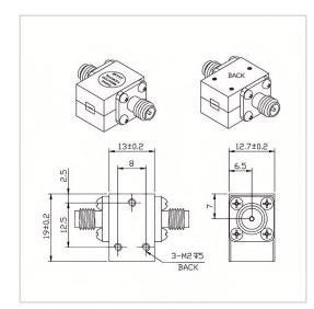
RF Solution offer a wide selection of Coaxial Isolator for global customers. TG1319CS is a Coaxial Isolator in Frequency Range of 6.0~12.0 GHz. It is made of high quality materials under a high standard, the Bandwidth Max of this product is 40%, Insertion Loss Max is 0.30~0.60 dB and Isolation Min is 15.0~23.0 dB. The component has a good working performance and stability, it is ideal for handling a Forward Power of 30 W.
