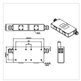
RF Solution offer a wide selection of Dual Junction Isolator for global customers. TG12060EN is a Dual Junction Isolator in Frequency Range of  $80\sim230$  MHz. It is made of high quality materials under a high standard, the Bandwidth Max of this product is  $5\sim30\%$ , Insertion Loss Max is  $0.80\sim2.20$  dB and Isolation Min is  $36.0\sim40.0$  dB. The component has a good working performance and stability, it is ideal for handling a Forward Power of 50/100 W.
