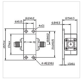
RF Solution offer a wide selection of Coaxial Isolator for global customers. TG1017CG is a Coaxial Isolator in Frequency Range of 19.0~31.0 GHz. It is made of high quality materials under a high standard, the Bandwidth Max of this product is 38%, Insertion Loss Max is 0.70~1.20 dB and Isolation Min is 20.0 dB. The component has a good working performance and stability, it is ideal for handling a Forward Power of 5/10 W.
