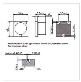
RF Solution offer a wide selection of Microstrip Circulator for global customers. SH0505-08 is a Microstrip Circulator in Frequency Range of 8.0~11.0 GHz. It is made of high quality materials under a high standard, the Bandwidth Max of this product is 100%, Insertion Loss Max is 0.60 dB and Isolation Min is 17.0 dB. The component has a good working performance and stability, it is ideal for handling a Forward Power of 10 W.
