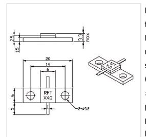
RF Solution offer a wide selection of Flanged Resistor for global customers. RFTXXN-60RM2006 is a Flanged Resistor in Capacitance of 2.9 PF@100 $\Omega$ . It is made of high quality materials under a high standard, the Resistance of this product is XX  $\Omega$ (10~2000 $\Omega$  Customizable), Resistance Tolerance is ±5% and Temperature Coefficient Max is 150 ppm/°C. The component has a good working performance and stability, it is ideal for handling a Power of 60 W.
