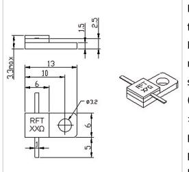
RF Solution offer a wide selection of Flanged Resistor for global customers. RFTXXN-60RM1306 is a Flanged Resistor in Capacitance of 2.9 PF@100 $\Omega$ . It is made of high quality materials under a high standard, the Resistance of this product is XX  $\Omega$ (10~2000 $\Omega$  Customizable), Resistance Tolerance is ±5% and Temperature Coefficient Max is 150 ppm/°C. The component has a good working performance and stability, it is ideal for handling a Power of 60 W.
