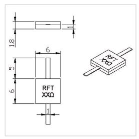
RF Solution offer a wide selection of Leaded Resistor for global customers. RFTXXN-60RM0606 is a Leaded Resistor in Capacitance of 2.9 PF@100 $\Omega$ . It is made of high quality materials under a high standard, the Resistance Range of this product is XX  $\Omega$  (10-3000 $\Omega$  Customizable), Resistance Tolerance is  $\pm 5\%$  and Temperature Coefficient Max is 150 ppm/°C. The component has a good working performance and stability, it is ideal for handling a Power of 60 W.
