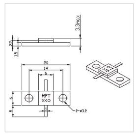
RF Solution offer a wide selection of Flanged Resistor for global customers. RFTXXN-30RM2006 is a Flanged Resistor in Capacitance of 2.9 PF@100 $\Omega$ . It is made of high quality materials under a high standard, the Resistance of this product is XX  $\Omega$  (10~2000 $\Omega$  Customizable), Resistance Tolerance is  $\pm 5\%$  and Temperature Coefficient Max is 150 ppm/°C. The component has a good working performance and stability, it is ideal for handling a Power of 30 W.
