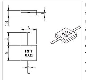
RF Solution offer a wide selection of Leaded Resistor for global customers. RFTXXN-30RM0606 is a Leaded Resistor in Capacitance of 2.9 PF@100 $\Omega$ . It is made of high quality materials under a high standard, the Resistance Range of this product is XX  $\Omega$  (10-3000 $\Omega$ Customizable), Resistance Tolerance is ±5% and Temperature Coefficient Max is 150 ppm/°C. The component has a good working performance and stability, it is ideal for handling a Power of 20 W.
