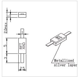
RF Solution offer a wide selection of Leaded Resistor for global customers. RFTXXN-20RM2550 is a Leaded Resistor in Capacitance of 2.4 PF@100 $\Omega$ . It is made of high quality materials under a high standard, the Resistance Range of this product is XX  $\Omega$  (10-3000 $\Omega$  Customizable), Resistance Tolerance is  $\pm 5\%$  and Temperature Coefficient Max is 150 ppm/°C. The component has a good working performance and stability, it is ideal for handling a Power of 20 W.
