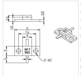
RF Solution offer a wide selection of Flanged Resistor for global customers. RFTXXN-20RM1104 is a Flanged Resistor in Capacitance of 2.3 PF@100 $\Omega$ . It is made of high quality materials under a high standard, the Resistance of this product is XX  $\Omega$ (10~3000 $\Omega$  Customizable), Resistance Tolerance is ±5% and Temperature Coefficient Max is 150 ppm/°C. The component has a good working performance and stability, it is ideal for handling a Power of 20 W.
