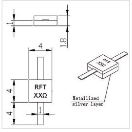
RF Solution offer a wide selection of Leaded Resistor for global customers. RFTXXN-20RM0404 is a Leaded Resistor in Capacitance of 2.3 PF@100 $\Omega$ . It is made of high quality materials under a high standard, the Resistance Range of this product is XX  $\Omega$  (10-3000 $\Omega$  Customizable), Resistance Tolerance is  $\pm 5\%$  and Temperature Coefficient Max is 150 ppm/°C. The component has a good working performance and stability, it is ideal for handling a Power of 20 W.
